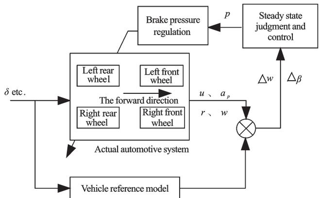
Figure 3 Diagram of Vehicle Stability Adaptive Control
