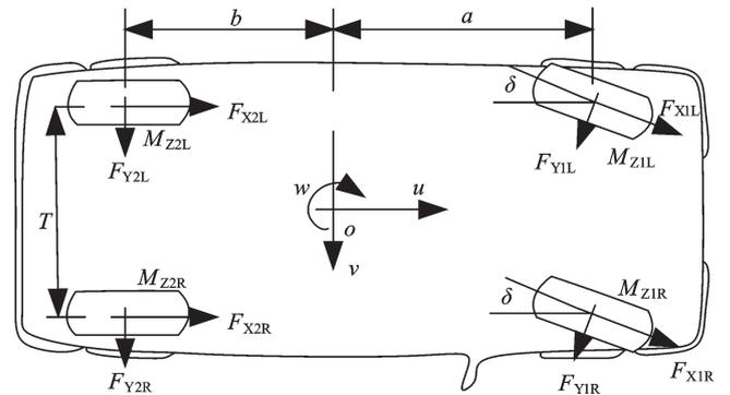
Figure 1 Schematic Vehicle with Seven Freedoms
