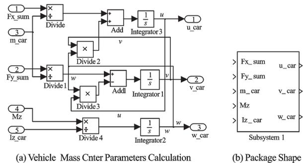
Figure 2 Block of Vehicle Centric Parameter Calculation
